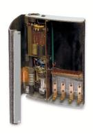
In August 1957, Labor W showed its first wireless microphone at a tradeshow in Frankfurt. It had been developed together with broadcaster NDR and had, under ideal conditions, a range of up to 100 m and an operating time of up to five hours. Pictured is the wireless transmitter, which still used a tube and consequently needed five batteries. A handheld microphone was plugged in at the transmitter top.
